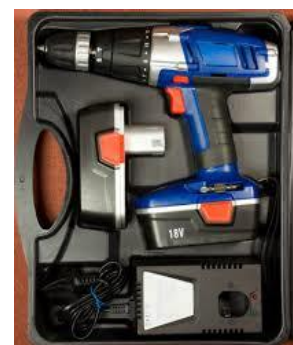
Figure 1, Example of lithium batteries packed with equipment, in the original packaging.
